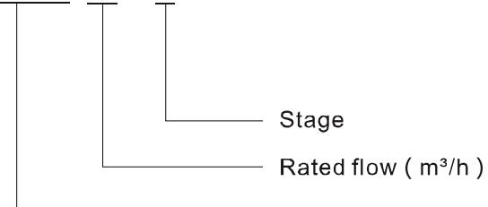
Vertical multistage intelligent variable frequency pump (F : Flow passage component : stainless steel 304 or 316L, general type omitted)
