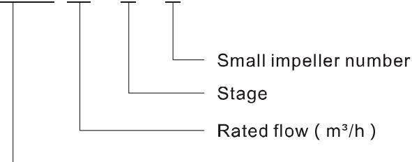
Vertical multistage intelligent variable frequency pump (F : Flow passage component : stainless steel 304 or 316L, general type omitted)
